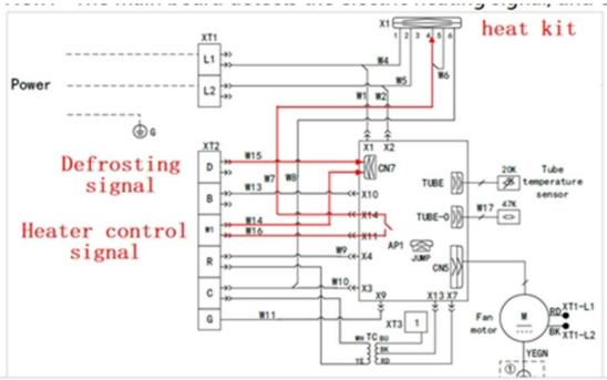
2. If no electric heat kit is installed, simply remove the wires from X11 and X14.
