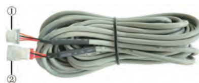
Fig. 25: Schematic diagram of connection wire: Connect terminal ① with wired controller CN1; connect terminal ② with the terminal ④ of patch cord
