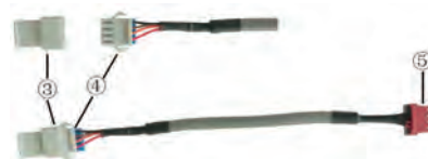
Fig. 26: Schematic diagram of patch cord: Terminal ③ is the protection terminal; connect terminal ④ to the terminal ② of connection wire; connect terminal ⑤ to the terminal of wired controller of air conditioner
