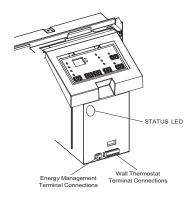
Fig. 21 – Terminal Connector and Status LED Location
