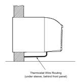
Fig. 19 – Proper Wire Routing
