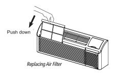
Fig. 27 – Removing and Replacing Air Filter
