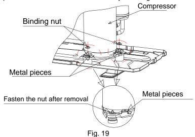
When installing the unit, metal pieces for transportation must be removed. Then fasten the binding nuts again and wrap back soundproofing cotton. If unit runs with metal pieces fitting on,
