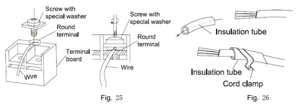
(3). How to fix connection cord and power cord by cord clamp
