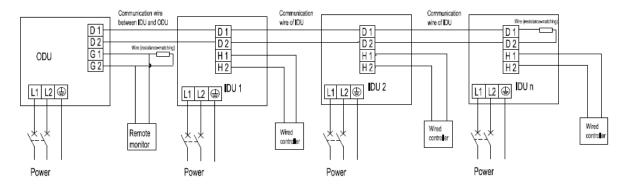
Fig.27 a Connection of power cord and communication wire for IDU and one ODU
