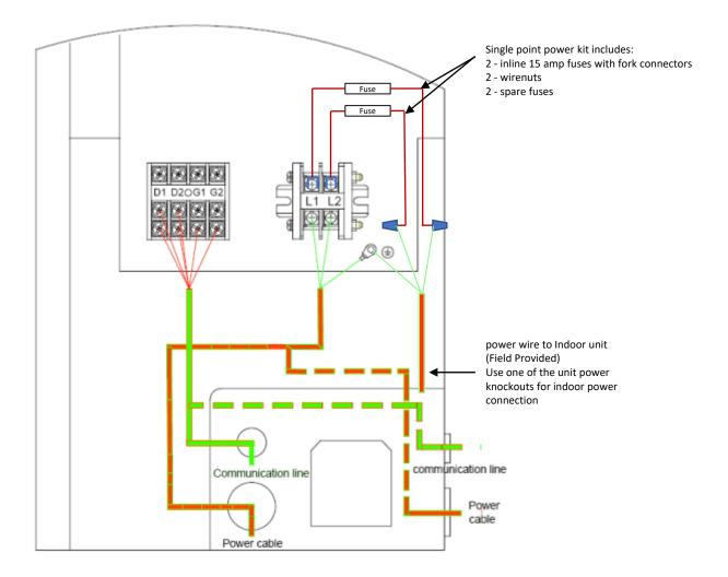
Control wire and power wire should be run in separately to avoid communication interference Outdoor unit MCA and MOCP values do not need to be adjusted when using this kit 3. Install fork connectors on inline fuse to L1 and L2 as shown
