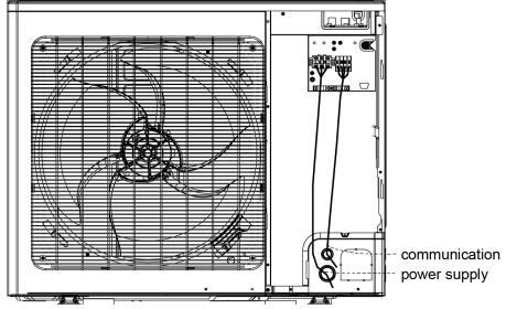
Fig. 22 Engineering Wiring View of GMV-24WL/C-T(U), GMV-28WL/C-T(U)
