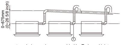
① - drainage pipes assembled by T-shaped joints
