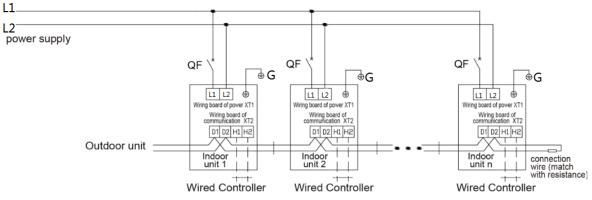
Note: indoor unit quantity n is according to the outdoor unit capacity.
