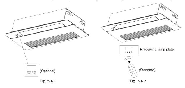
2) Both IDU and wired controller are equipped with signal receiver, and available for wireless control respectively.
