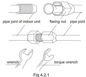
Torque for tightening nut
