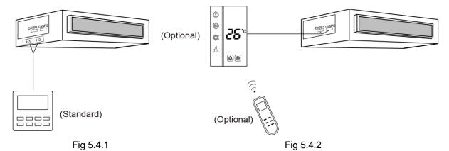
2) Fig 5.4.2 shows the installation of remote controller.
