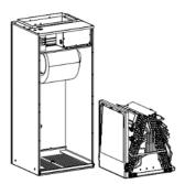
Evaporator Coil & Condensate Drain Pan
