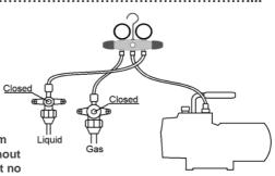
Recommend attaching micron gauge directly to the vacuum pump to test and verify it is capable of reaching 50-100 microns or less, before starting evacuation process. If this level of vacuum cannot be reached during the test, replacing the vacuum pump oil or vacuum pump itself may be necessary to achieve the 500 micron or less vacuum required.
