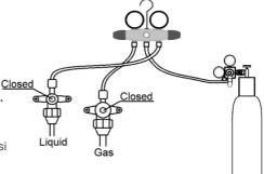
Recommend first pressurizing refrigerant lines to 100 psi with the use of dry nitrogen, then continuing to a minimum of 500 psi if no leaks are found to be present.
