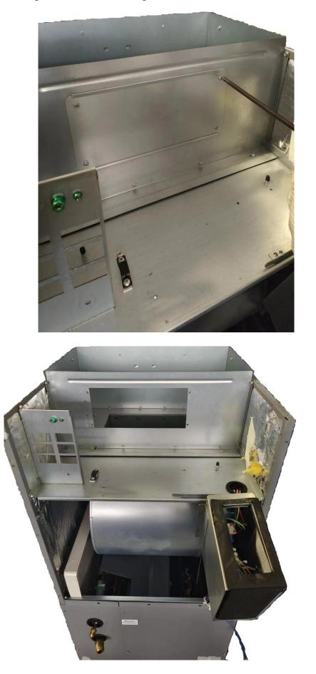
4. Install the electric heater in the position of the metal plate removed at Step 3. (Note:There are two holes underneath. They are used to fix the bracket of the electric heater.)
