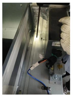
3. Remove the metal plate at the mounting holes of the electric heater.
