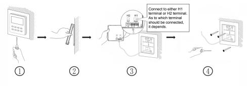
Fig. 24 Disassembly diagram for wired controller
