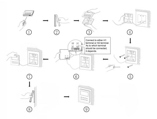
Fig. 23 Installation diagram for wired controller
