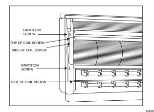
Fig. 15 – Location of Fan Assembly Screws on Opposite Side
