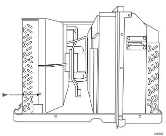
Fig. 36 – Location of Shroud to Coil Screw (Vent Door Side)
