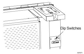
Fig. 51 – Dipswitch Location on Unit
