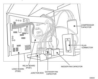
Fig. 49 – Location of Components Inside Control Box
