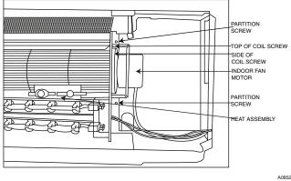
Fig. 14 – Location of Fan Assy. Screws on Fan Motor Side
