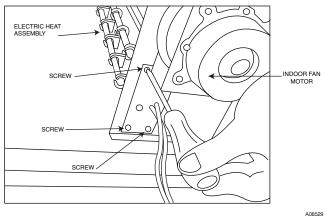
Fig. 17 – Location of Heater Assembly Screws (Fan Motor Side)
