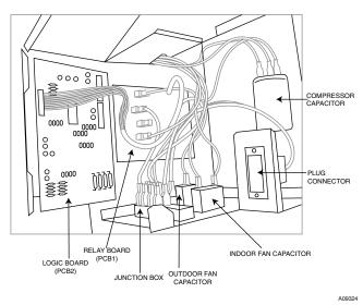
Fig. 22 - Location of Components Inside Control Box
