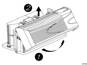
Fig. 3 – Removal of Front Panel
