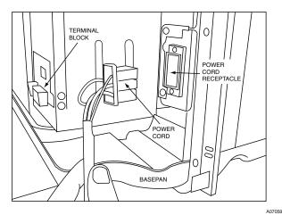
Fig. 5 - Plug Assembly on Hardwire Units
