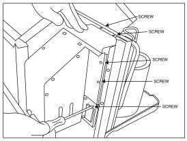
Fig. 12 – Remove 5 Screws from Electrical Box
