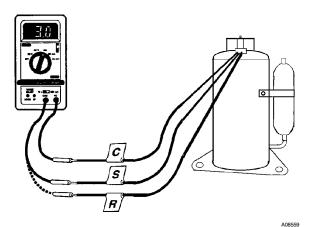
Fig. 39 – Shorted/Open Windings Test
