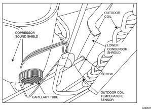
Fig. 35 – Location of Shroud to Coil Screw (Compressor Side)
