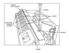
Fig. 9 – Removal of Screws from Top Plate
