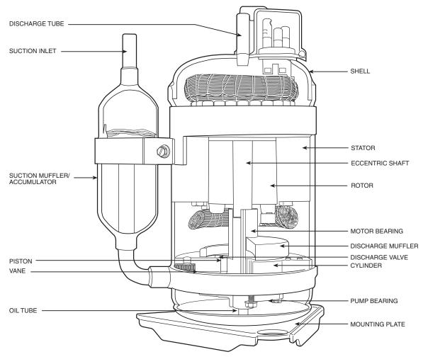
Fig. 37 - Rotary Compressor Components
