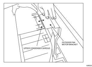
Fig. 31 - Push Condenser Shroud from Fan Motor Bracket
