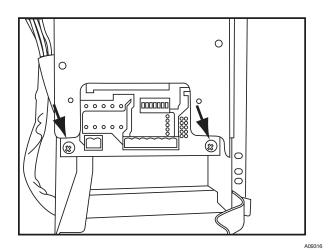
Fig. 26 – Location of Screws Holding Control Board to Control Box
