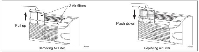
Fig. 64 – Removing and Replacing Air Filter
