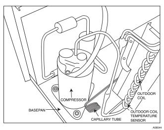
Fig. 48 – Location of Outdoor Coil Sensor
