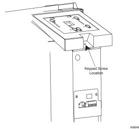
Fig. 19 - Keypad Screw Location
