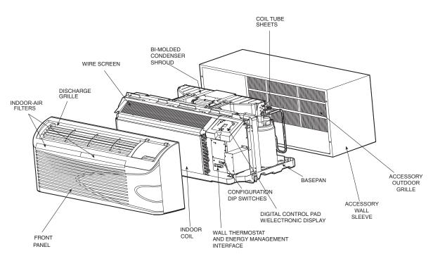
Fig. 61 – Typical GA series PTAC System
