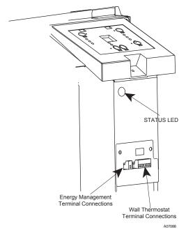
Fig. 53 - Terminal Connector and Status LED Location
