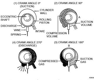
Fig. 38 – Rotary Compressor Compression Process
