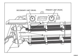
Fig. 43 – Limit Switch Location
