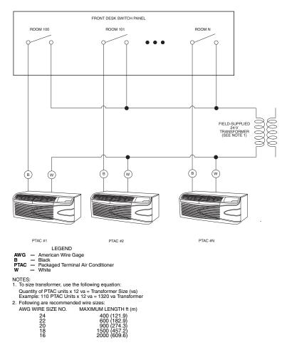
Fig. 59 – Energy Management Wiring Schematic
