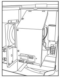
Fig. 25 – Screw Location in Front Cover
