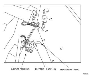
Fig. 13 – Heater Limits, Electric Heat, and Indoor Fan Motor Plugs
