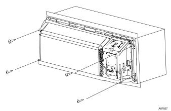
Fig. 7 – Location of Wall Sleeve Screws
