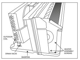
Fig. 18 – Location of Heater Assembly Screws (Opposite Side)
