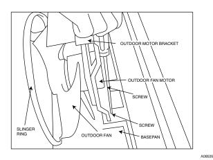
Fig. 33 – Location of Fan Motor Bracket Screws
