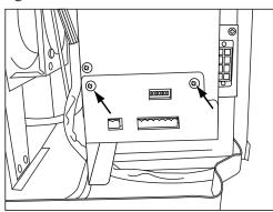
Fig. 23 – Location of Control Box Cover Screws
