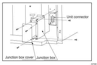
Fig. 4 – Removal of Junction Box Cover
