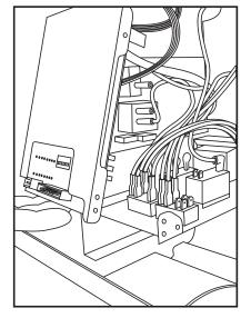
Fig. 27 – Pull Control Box Away From Bottom
