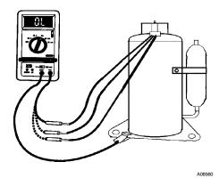
Fig. 40 – Grounded Windings Test
