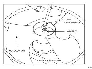
Fig. 34 – Remove 10 mm Nut on Fan Motor Shaft
