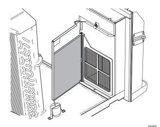
Fig. 45 – Condensate Drain Valve
