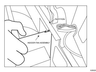
Fig. 16 – Separate Indoor Fan Assembly from Partition
