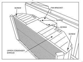
Fig. 29 – Location of Attachment Screws on Top of Condenser Shroud
