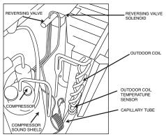
Fig. 41 – Reversing Valve Solenoid and Outdoor Temperature Sensor
