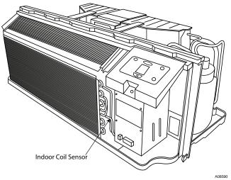
Fig. 47 – Location of Indoor Coil Sensor
