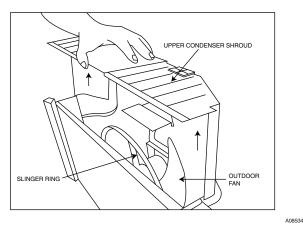
Fig. 32 - Removal of Upper Condenser Shroud
