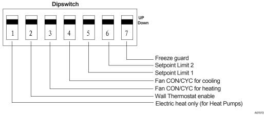
Fig. 52 – Dip Switches
