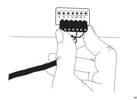
Fig. 56 - Terminal Connector Removal and Replacement
