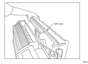
Fig. 10 – Removing Top Plate from Unit
