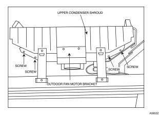
Fig. 30 – Location of Screws Connecting Shroud
