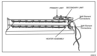
Fig. 44 - Heater Coil (Removed)
