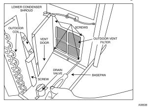
Fig. 65 – Removal of Outdoor Vent Filter Screws
