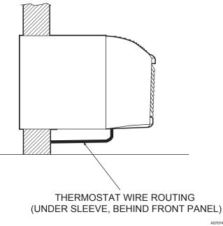
Fig. 54 – Proper Wire Routing Beneath Unit
