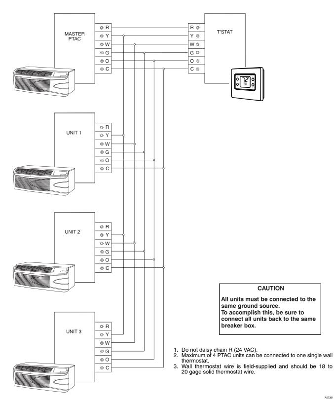
Fig. 58 – Typical Wiring Schematic for Multiple PTAC Units Connected to a Single Wall Thermostat
