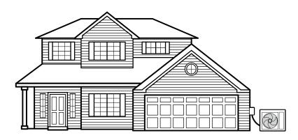
The main power is supplied to the outdoor unit. System must be on a single dedicated circuit. Use appropriate wire size and circuit breaker (or fuse) size for proper system overcurrent protection. Follow all local building codes and NEC (National Electrical Code) regulations.
